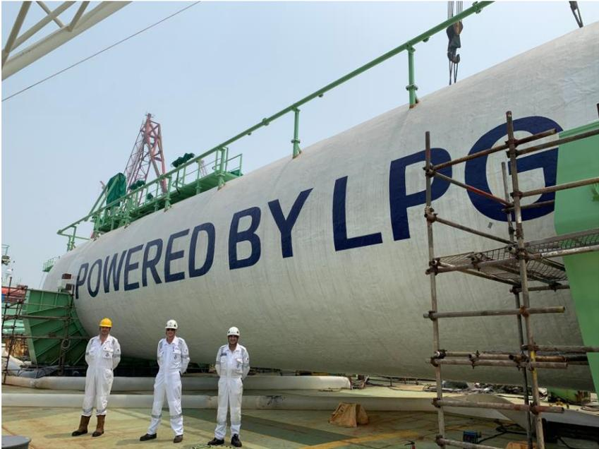
Figure 100: Pressurized LPG storage tanks installed on the *BW Gemini*, IMO no. 9703007 (source: [BW LPG](#))
