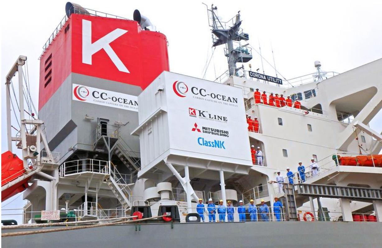
Figure 130: MHI absorption carbon capture system installed as part of CC-Ocean project (source: MHI)
