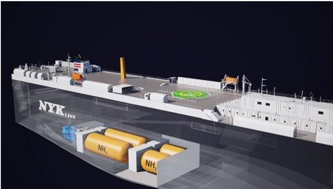
Figure 123: NYK Line ammonia-fuel ready LNG-fueled car carrier concept (source: NYK)
