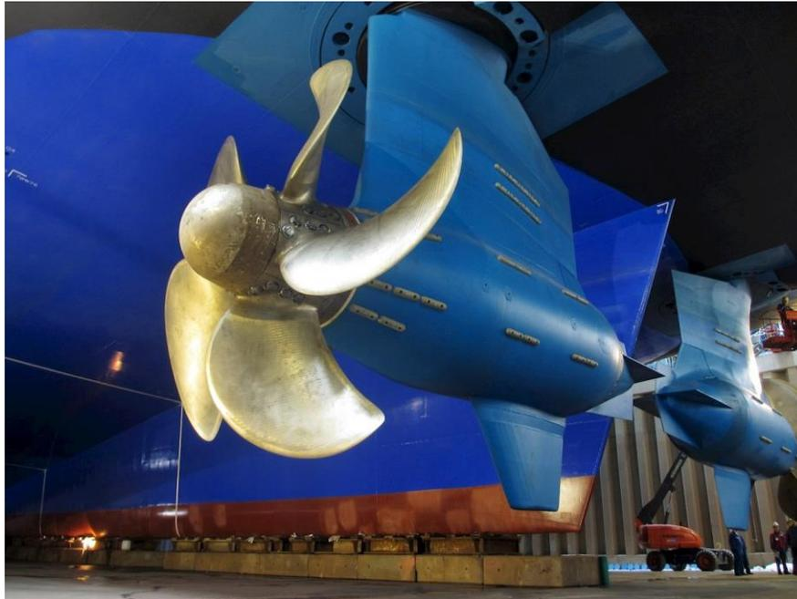
Figure 25: ABB's Azipod® steering and propulsion system (source: ABB)
