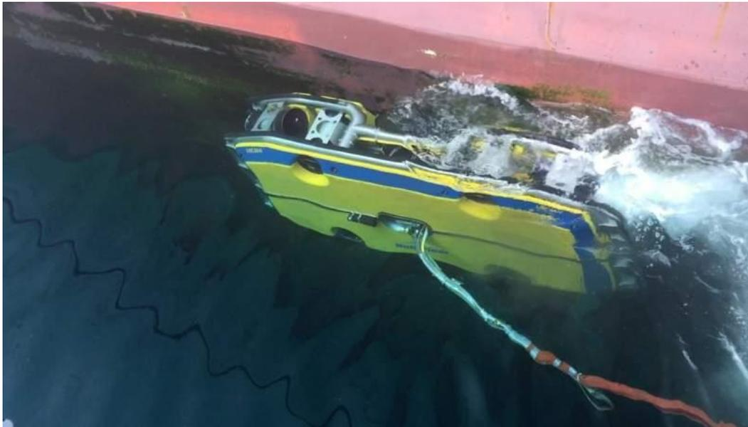
Figure 14: HullWiper's underwater hull cleaning technology uses adjustable seawater jets under variable pressure as the means of cleaning (Source: HullWiper [B6])
