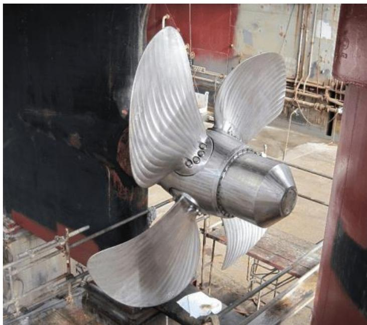
Figure 23: CPP system installed on Washington State Ferries vessels (source: [travelswithtowhee.com](#))
