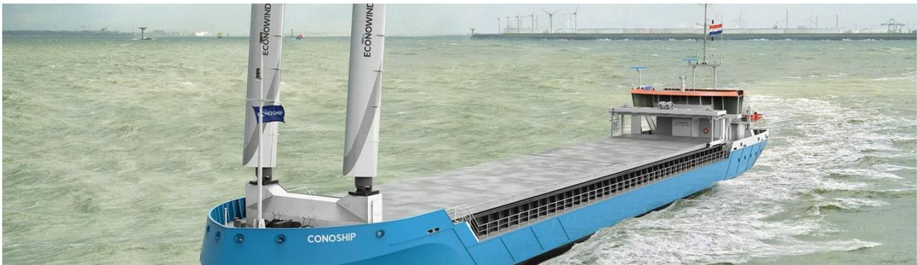
Figure 125: Conoship CIP3600 concept with diesel-electric propulsion (source: [Conoship International](#))
