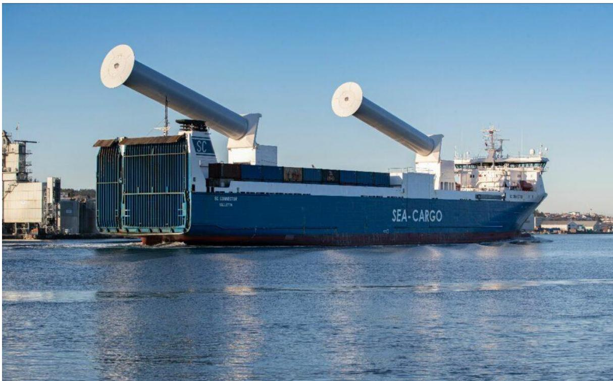
Figure 85: SC Connector RoRo with Norsepower folding rotor sails (source: Norsepower)
