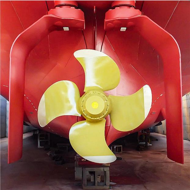
Figure 33: Kamome Gate Rudder® for increasing thrust and reducing rudder resistance (source: Kamome Propeller)
