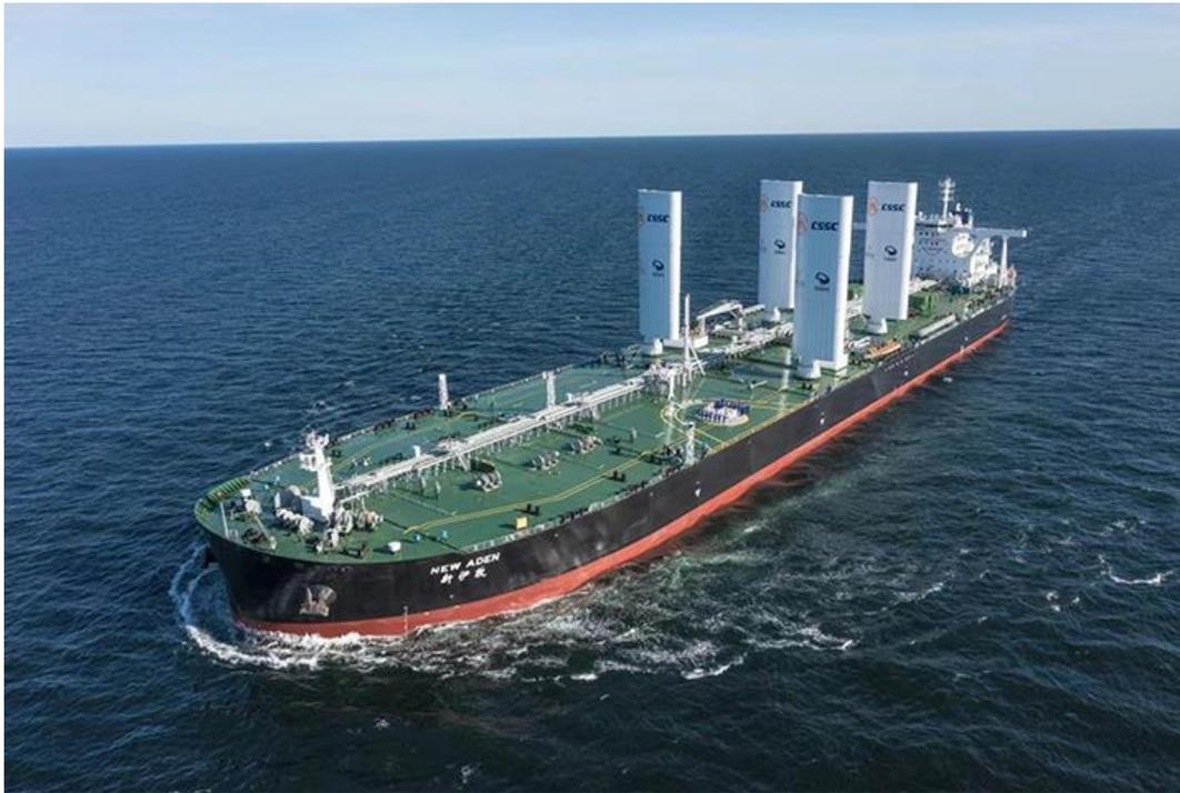
Figure 88: VLCC *New Aden* (IMO no. 9912000) fitted with four 40-meter wingsails (source: [Marine Log](#))
