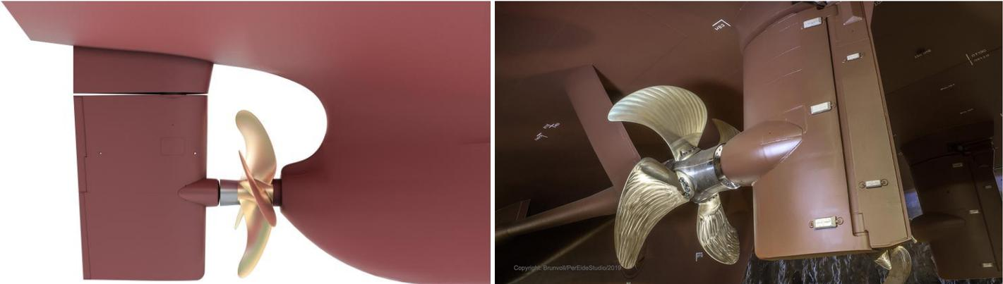
Figure 34: Kongsberg Promas propulsion system with costa bulb (left, source: Kongsberg [B18]) and Brunvoll integrated costa bulb (right, source: Brunvoll [B19])
