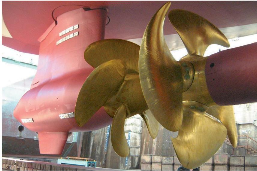
Figure 24: CRP mounted separately on azimuthing pod and stern drive (source: ABB)
