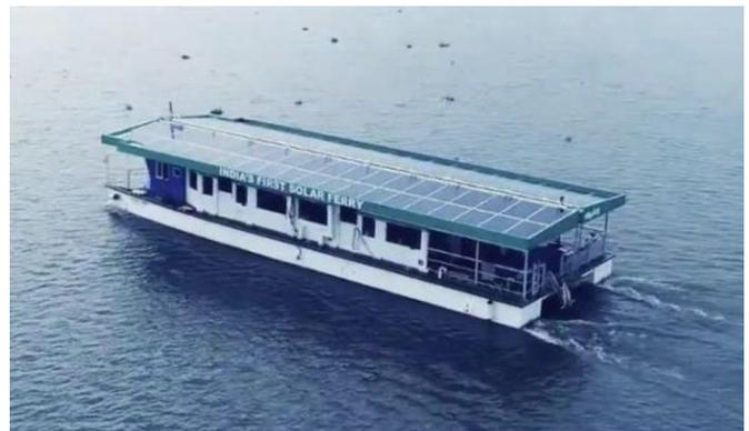
Figure 94: *Aditya* passenger ferry with 20 kW of solar capacity (source: ewnsnews.com)
