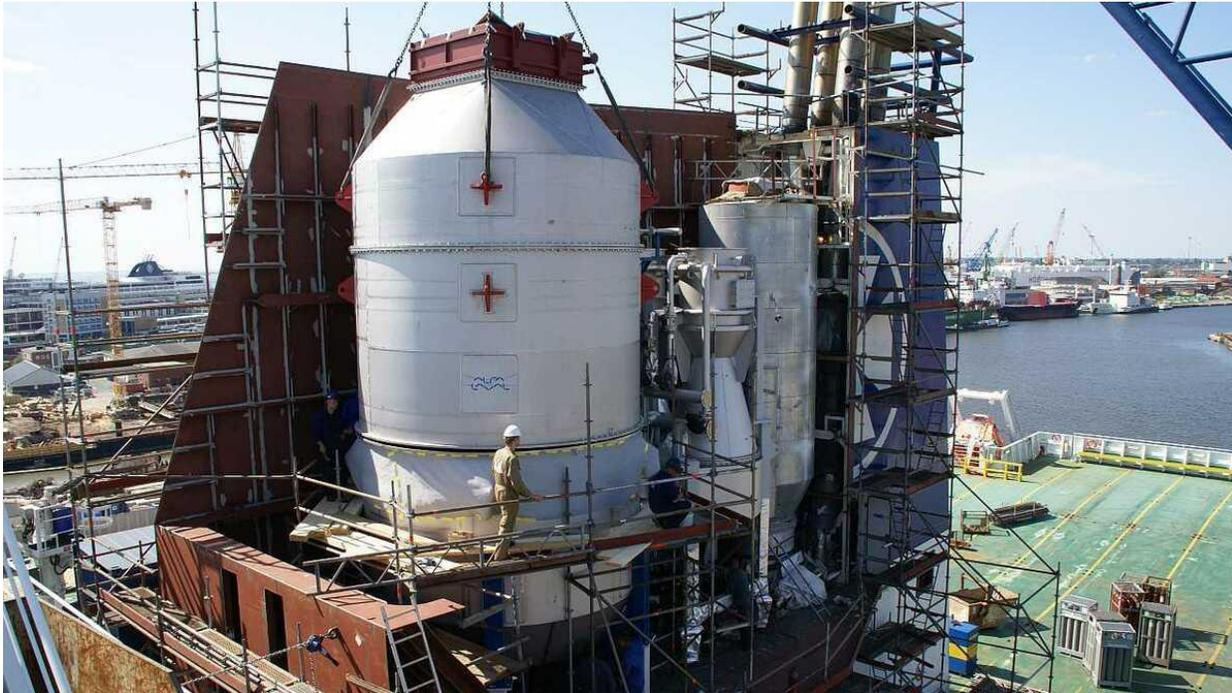
Figure 129: Alfa Laval has tested its SOx scrubber technology to absorb CO<sub>2</sub> (source: Alfa Laval via [rivieramm.com](https://rivieramm.com))
