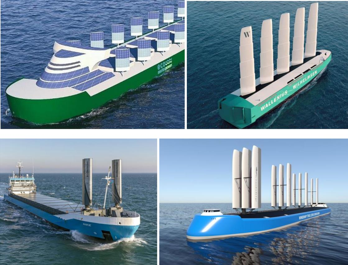
Figure 87: Various rigid wingsail technologies, clockwise from upper left: Aquarius MRE (Eco Marine Power), Orcelle Wind (Wallerenius Wilhelmsen), Wingship (Wingship), and Ventifoil retrofit (Econowind)
