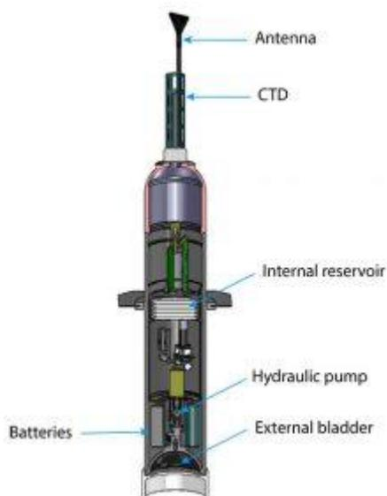
While there are a few different styles of Argo float, they mostly follow the same design – a cylinder a little over 3ft long. A set of sensors (called CTD) at the top collect conductivity (salinity), temperature, and pressure (depth) measurements. Inside the cylinder, pumps and reservoirs allow the float to sink slowly to a depth of 1.24 miles (2000m) or more and rise again to transmit data.
